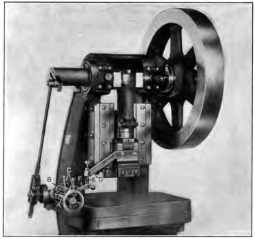
Fig. 2. Inclinable Press having a Rack-operated Roll Feed
